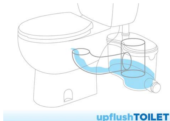
Figure 2. Internal water flow of vertical toilet [3]
