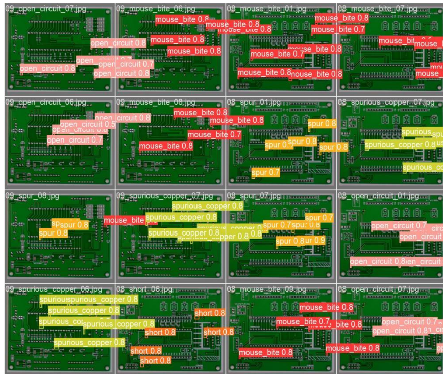
Fig. 4 Five types of PCB defects
