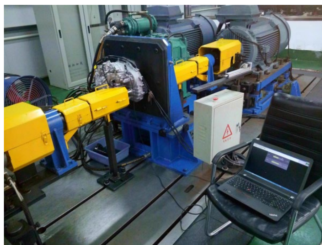
Figure 5. Real-time data processing verification of vehicle transmission
