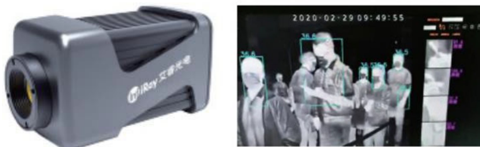
Figure 1. Arrow's thermal imager and monitoring interface
