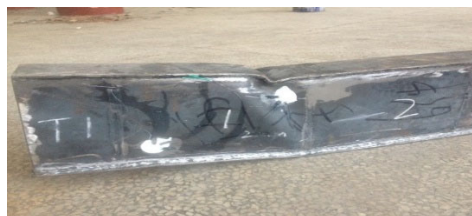
Fig. 13 Picture of web plate buckling under shear action of steel box girder
