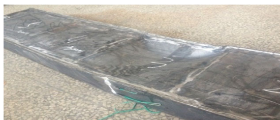
Fig. 18 Partial enlarged drawing of instability position of test beam
