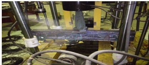
Fig. 12 Test model of ultimate bearing capacity under shear force of steel beam
