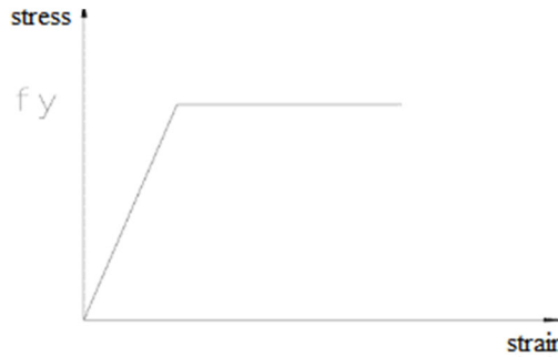
Fig. 2 Stress-strain curve of the material
