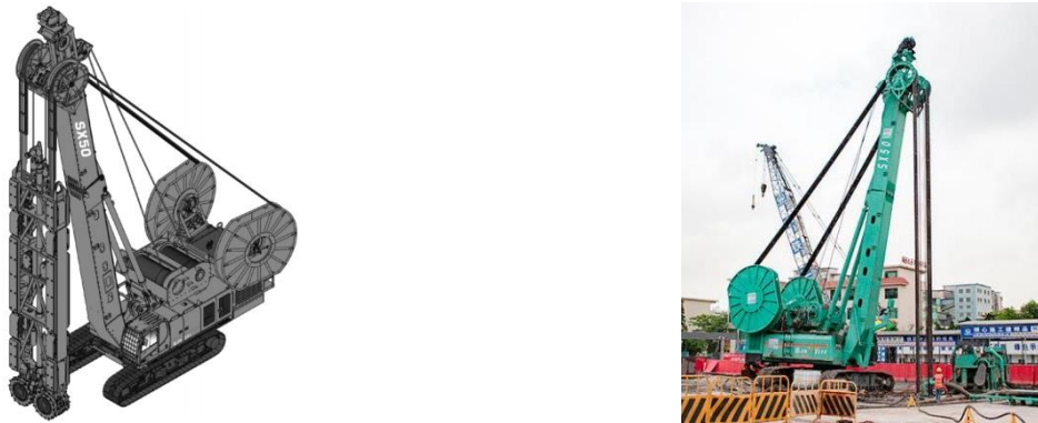
Figure 4 SX50 double wheel slot milling machine made in China[12]
