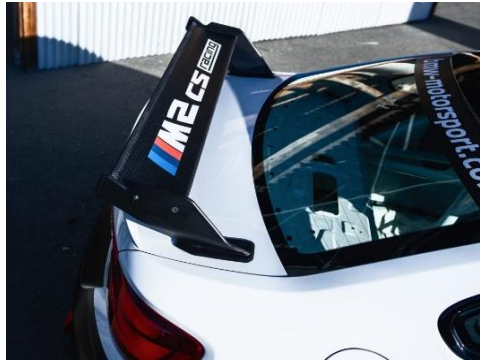
Fig. 5 The M2CS Adjustable rear wing
