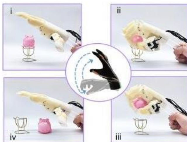
Figure 16. A robotic hand controlled by P-HCF sensors to (i) open (ii) grasp the object (iii) move (iv) drop the object [13]
