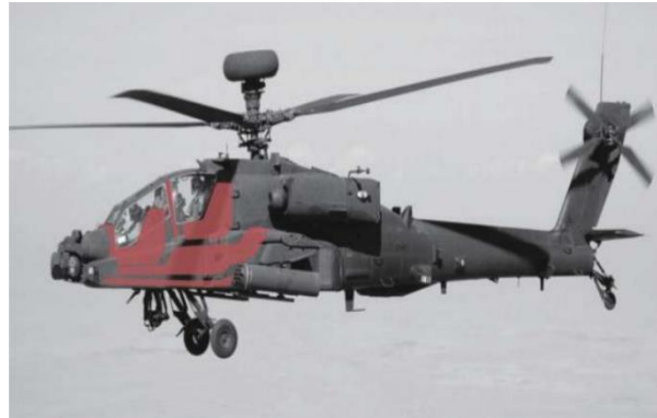
Figure 1. Cockpit protective armor of Apache gunship [3]
