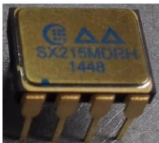
Figure 13. Domestic high-precision operational amplifiers for astronautics [15]
