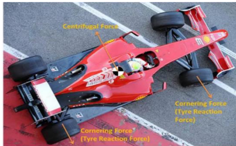
Figure 4. Forces Exerting on the Formula 1 vehicle while turning
