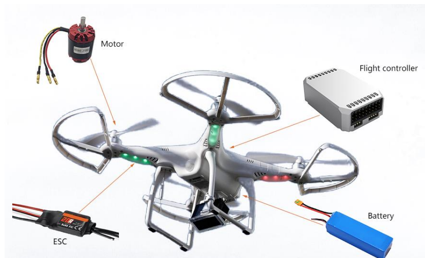
Fig. 1 UAV's basic hardware structure (Photo/Picture credit: Original)
