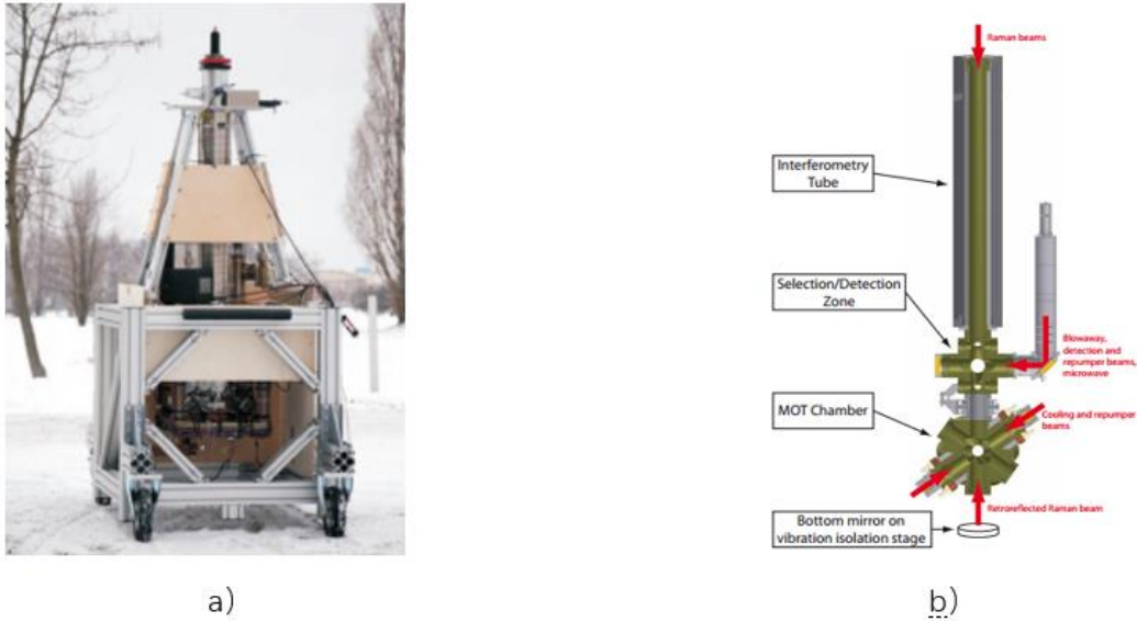
Fig. 7 Portable atomic interferometry gravimeter [14].
