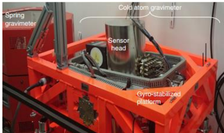
Fig. 6 Shipborne atomic interferometry gravimeter [10].
