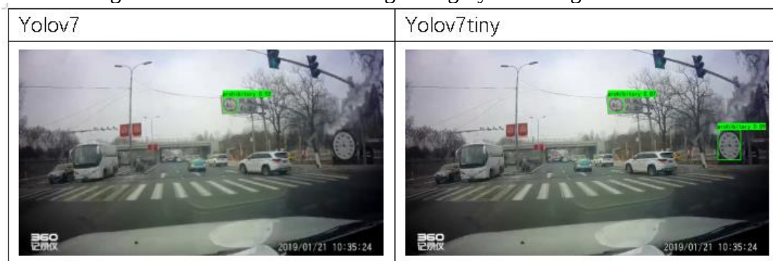
Fig. 6 Visualization of detection results of YOLOV7 and YOLOV7-tiny models
