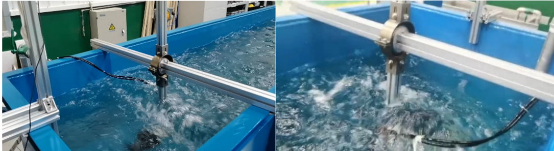
Figure 2. Real propeller open water test
