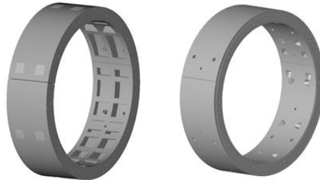
Fig 4. Concrete segment and steel segment.
