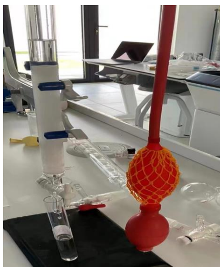
Fig. 9 Column chromatography apparatus with a silica gel column, a pump for increasing the pressure and a test tube holding the solution dropping down.
