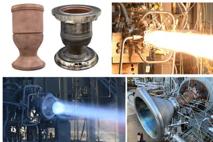
Fig. 10 Examples of fully AM thrust chamber assemblies hot-fire tested at NASA MSFC including injectors, combustion chambers, and channel-cooled nozzles, including L-PBF GRCop-84, L-PBF GRCop-42, bimetallic L-PBF and DED, and LP-DED NASA HR-1 [9]
