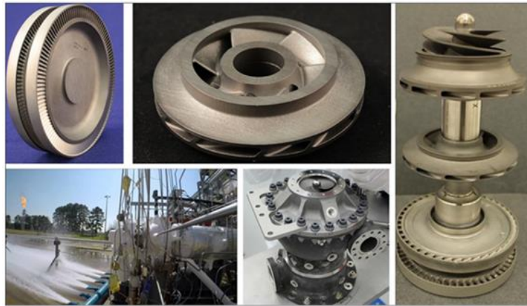
Fig. 7 Examples of liquid hydrogen and liquid oxygen turbopumps using AM at NASA MSFC [6,13]
