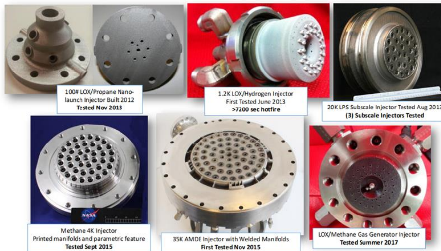
Fig. 4 Examples of injectors produced by MSFC of NASA using SLM technology [9]
