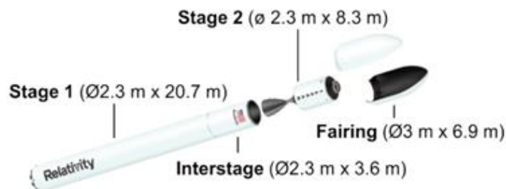
Fig. 8 The Terran 1 launch vehicle by Relativity makes use of 3D printing for practically all of the propulsion components and all of the primary structures [12].
