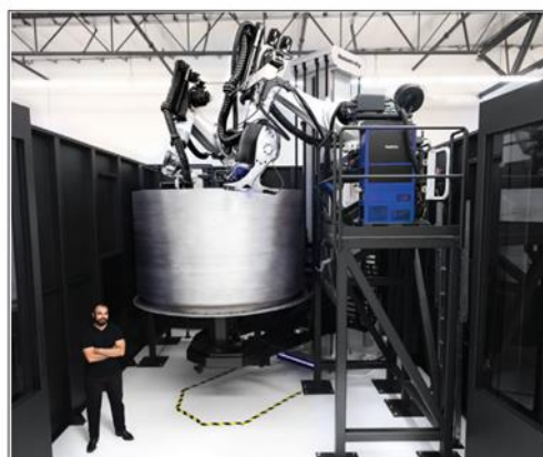
Fig. 9 Relativity's Stargate 3D Printing System producing a Terran 1 first stage tank section [12]
