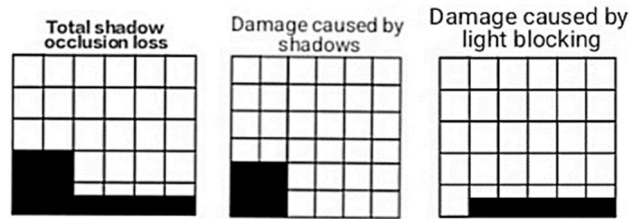
Figure 3. Classification of light reflection loss
