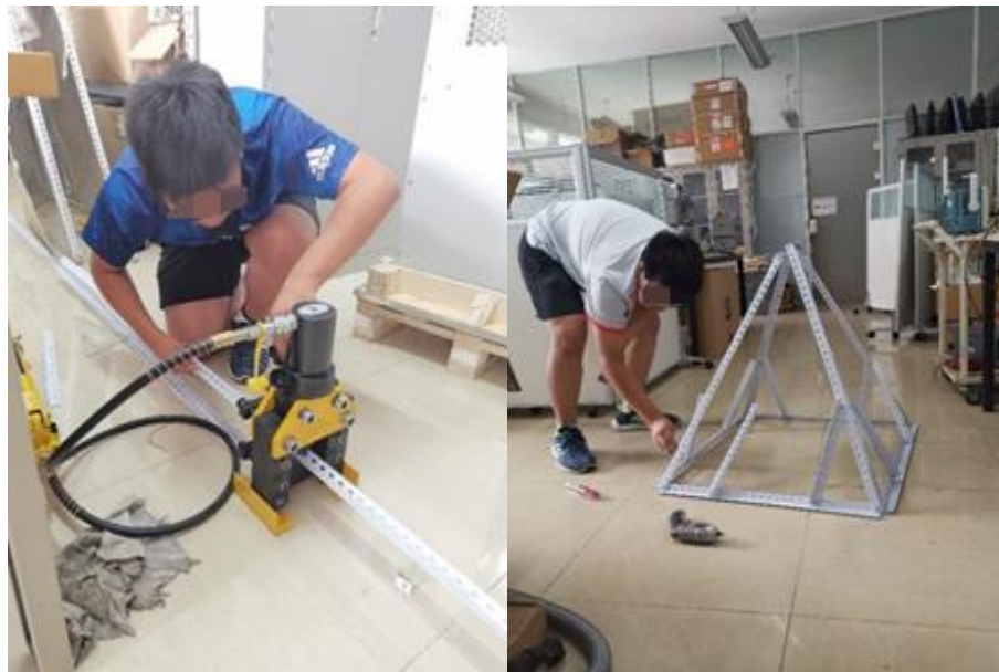
Figure 2. Preparing the angle iron with various lengths (left) and the assembly of the frame of the horn (right).
