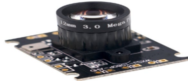
Fig.7 RER-USB4KHDR01 8 million camera module.
