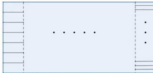
Figure 9. Method of arranging survey lines when all are oriented east-west.
