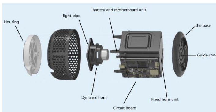
Fig 1. The inner structure of Xiaodu intelligent speakers (Photo/Picture credit: Original).
