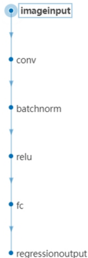
Figure 6. The structure of CNN regression prediction.
