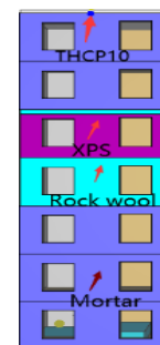
Figure 2. Diagram of external wall insulation construction
