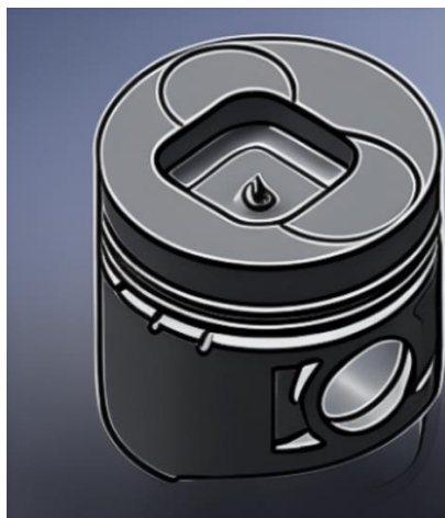
Fig. 1 Example of square bowl-type piston [2]
