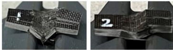
Fig. 4 Failure mode of interlaminar shear test under 800°C dry conditions
