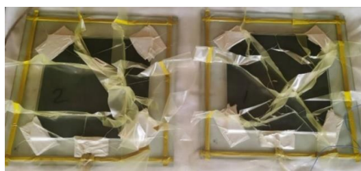
Fig. 1 The composite motherboard was vacuumed and cured in the oven.
