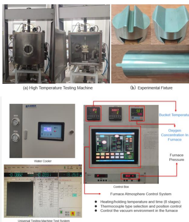
Fig. 2 High temperature test equipment and operating system diagram
