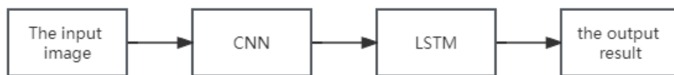
Fig. 4 The structure of the handwriting recognition model using LSTM (Photo/Picture credit: Original)
