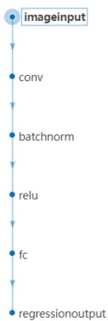
Figure 6. The structure of CNN regression prediction
