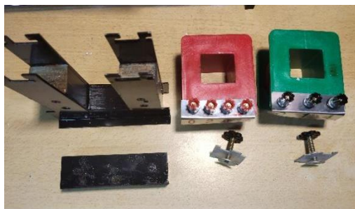
Fig 6. Removal of Top Device, Bar Yoke, and Both Side Coils.
