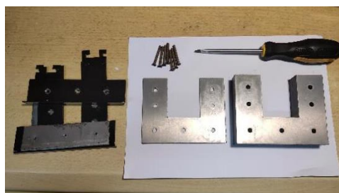
Fig 7. Screwdriver to screw out the screws of the U-core and separate the U-core.
