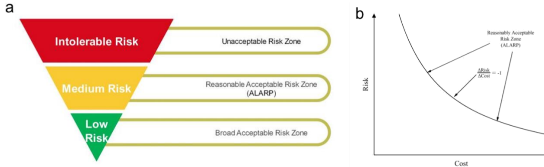
Figure 2: Schematic diagram of the risk assessment criteria. (a) ALARP criterion. (b) Cost-Risk Curve
