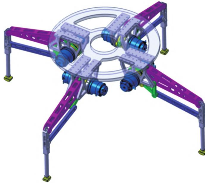
Fig. 5 Design form of bionic landing gear mechanism [9]
