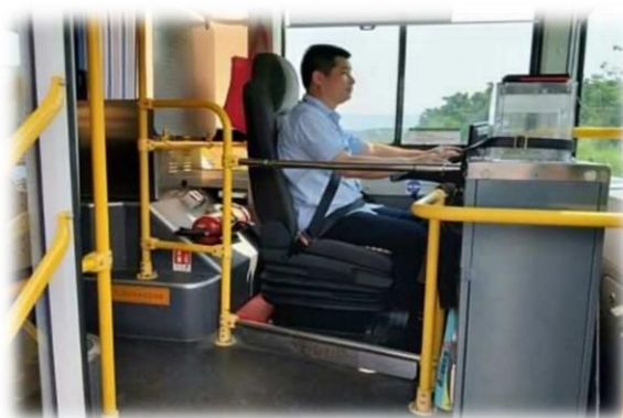
Fig 2. Driver's workspace in China - Before Improvement [5].
