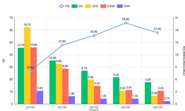
Fig. 3 Yield of gaseous components from DFA/CE pyrolysis
