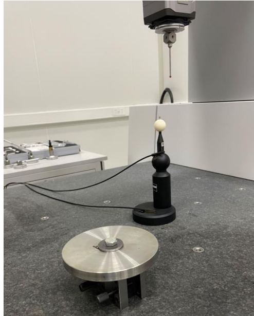
Figure 1. Schematic diagram of cylindricity measurement process based on CMM
