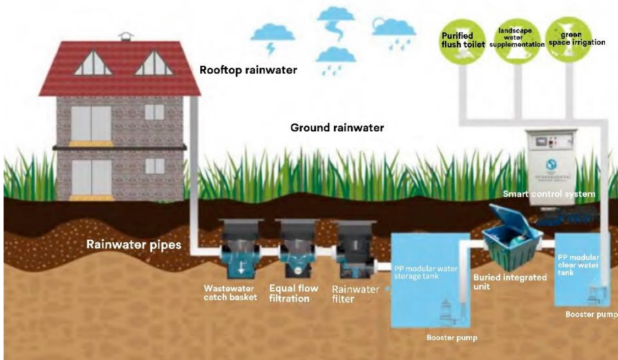
Fig. 1 Rainwater Recovery System [3]
