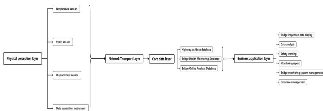
Fig. 4 Monitoring data processing flow charts
