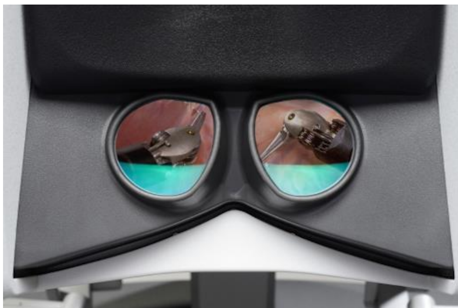
Fig. 1 High-performance on-site visual system of Da Vinci surgical system [5]
