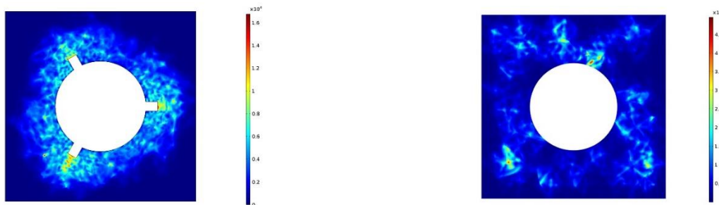
Figure 9 The length of the feeder is 30mm. The electric field die cutting plane at the center of the feeder and the center of the reservoir under working conditions
