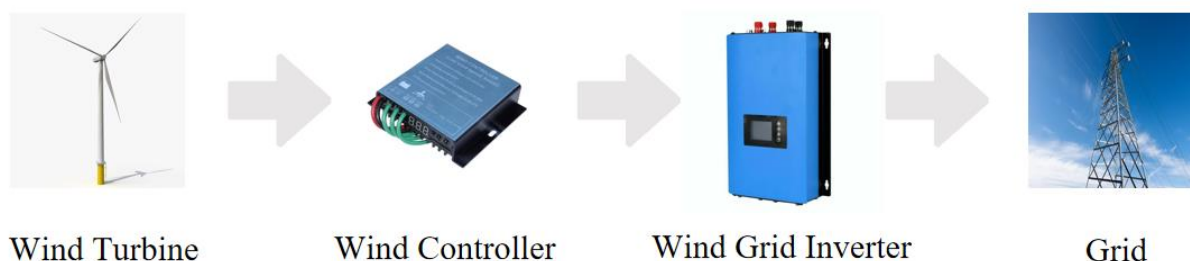
Fig. 1 Wind power grid connection (Photo/Picture credit: Original)
