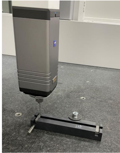
Figure 1. Schematic diagram of nonlinear planar distance measurement process based on CMM
