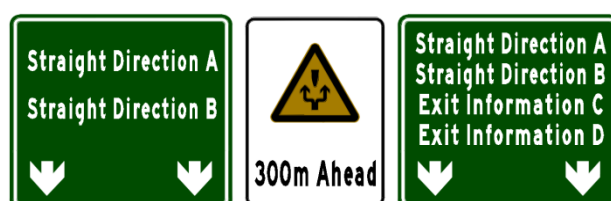
Fig. 3 Lane indication sign for the same-direction separated subgrade section (A, B, C and D are Location informations)
