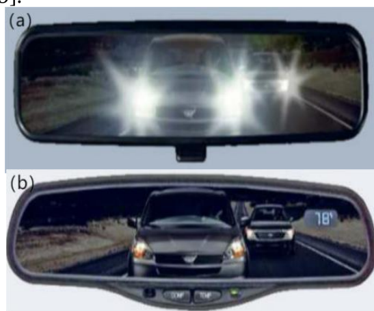
Figure 3 (a) Conventional mirror and (b) Modern antiglare mirror [19].
