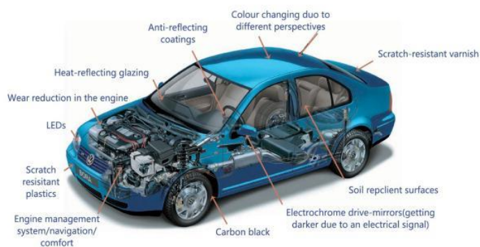
Figure 2 Development of materials used to construct a mid-sized car [9].
