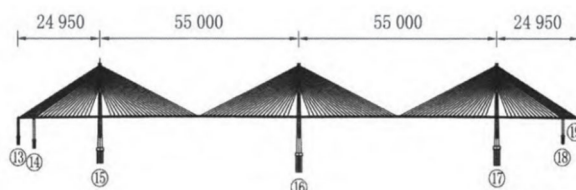
Figure 1. Elevation of the Pingtang Bridge
