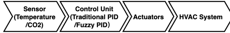
Fig. 1 The key components in a dynamic building climate control system. (Picture credit: Original)
