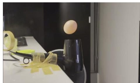
Figure 4. The ellipsoid over a vertical jet (Photo credit: Original).
