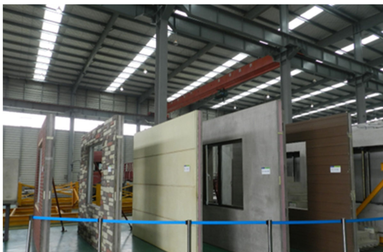
Figure 4. Concrete sandwich walls
