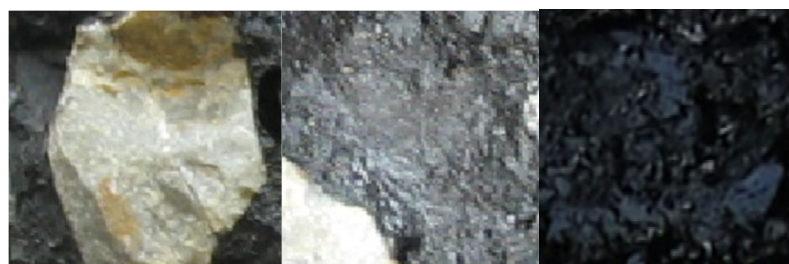
A. limestone fracture B. Interface fracture C. Asphalt layer fracture
