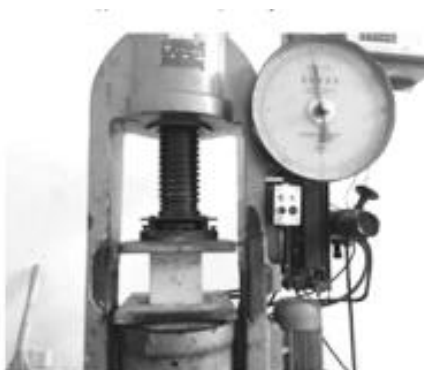
Figure 1. Compression testing machine
