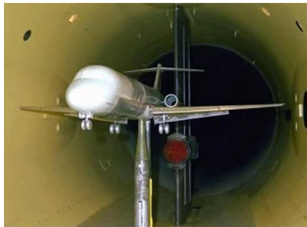
Fig. 8 Plane model in Wind tunnel
